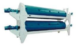
This machine is specially designed to separate broken rice from head rice based on the length of the input grain.
