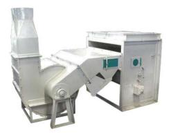
The main function of this machine is to separate husk from the shelled paddy. Shelled paddy is allowed to flow through a specially designed arrangement of flops.
