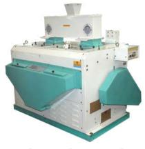
The machine is used to eliminate impurities like stone and clay particles from bran-free finished rice. The design of this machine is based on gravitational principles, and it is advised to install it after final polished rice.
