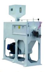
Silky Master Jumbo machines are the latest generation machines that give best quality polishing to rice and give a silky smooth finish to the rice grain. A special device provided with spray gun to get mist form with compressed air and water, it gives superior quality of smooth and silky rice.
